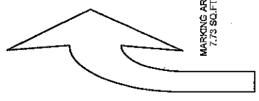
TYPE 2SR (RIGHT) TRAFFIC ARROW MIRROR IMAGE OF TYPE 2SL TRAFFIC ARROW (SHOWN AT REDUCED SCALE)
