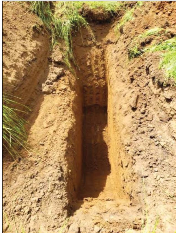
Photos TP-7: Test Pit TP-7 to approximately 9 feet in depth (below); Sample from bottom of exploration at 9 feet (left)
