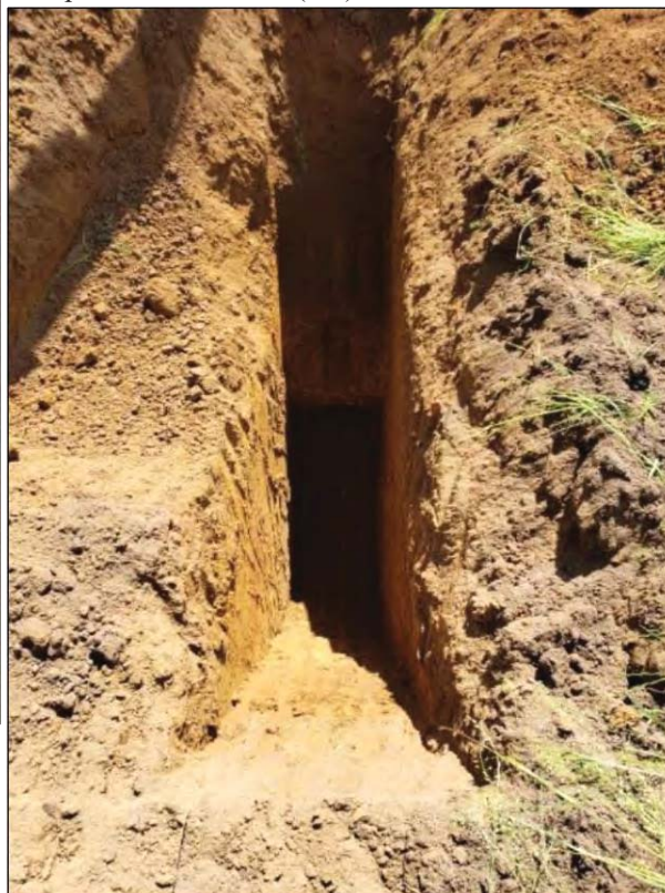
Photos TP-12: Test Pit TP-12 to approximately 12 feet in depth (below); Sample from bottom of exploration at 12 feet (left)
