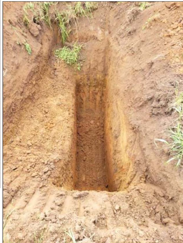
Photos TP-8: Test Pit TP-8 to approximately 9 feet in depth (below); Sample from bottom of exploration at 9 feet (left)
