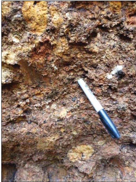
Photos TP-3: Test Pit TP-3 to approximately 7 feet in depth (below); in situ sample at approximately 5 feet below ground surface (left)
