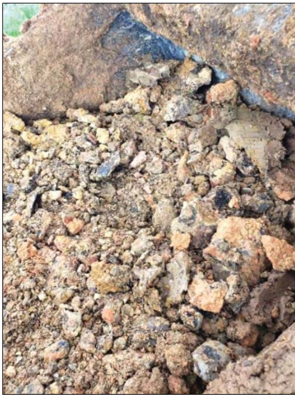
Photos TP-4: Test Pit TP-4 to approximately 8 feet in depth (below); Sample from bottom of exploration at 8 feet (left)
