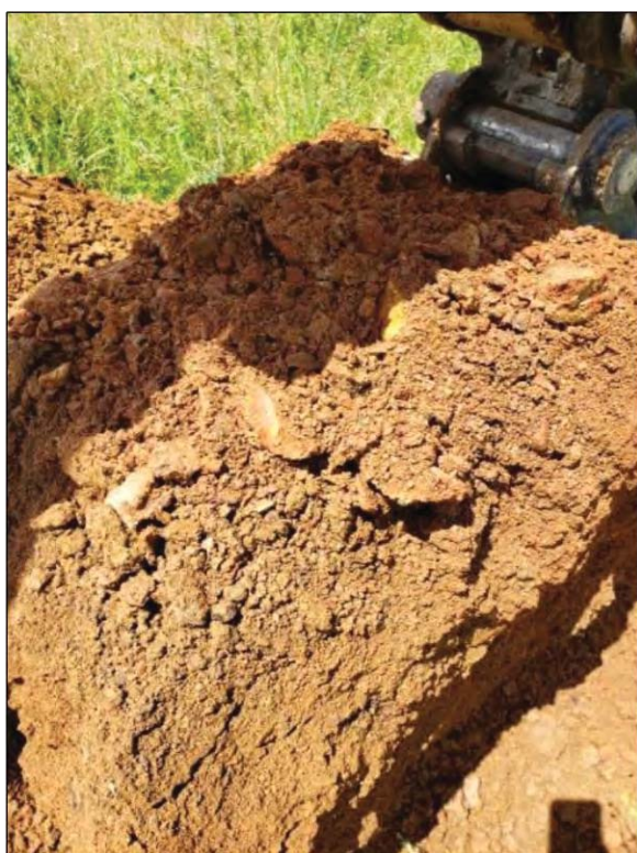
Photos TP-10: Test Pit TP-10 to approximately 7 feet in depth (below); Sample from bottom of exploration at 7 feet (left)
