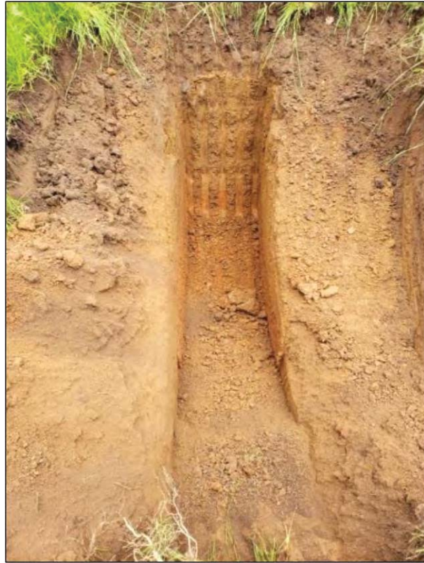
Photos TP-11: Test Pit TP-11 to approximately 6½ feet in depth (below); Sample from bottom of exploration at 6½ feet (left)
