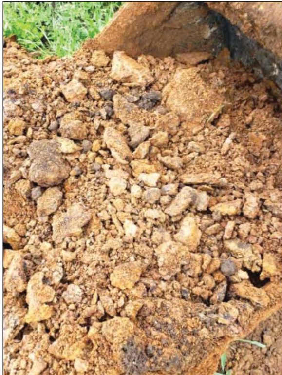
Photos TP-5: Test Pit TP-5 to approximately 6 feet in depth (below); Sample from exploration at approximately 6 feet (left)
