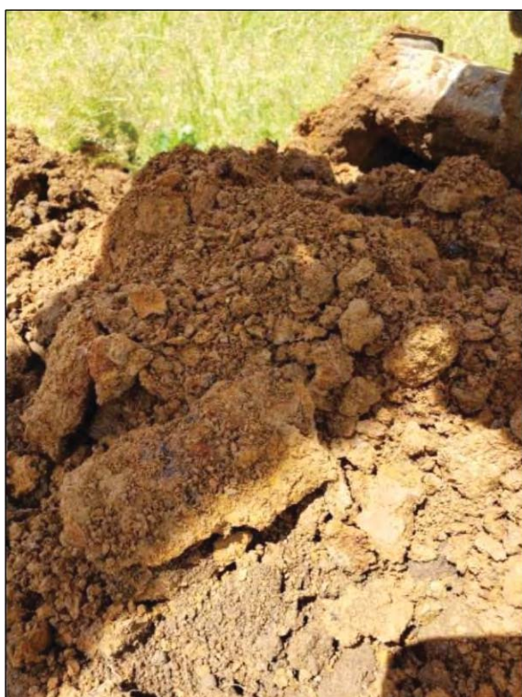
Photos TP-9: Test Pit TP-9 to approximately 7 feet in depth (below); Sample from bottom of exploration at 7 feet (left)
