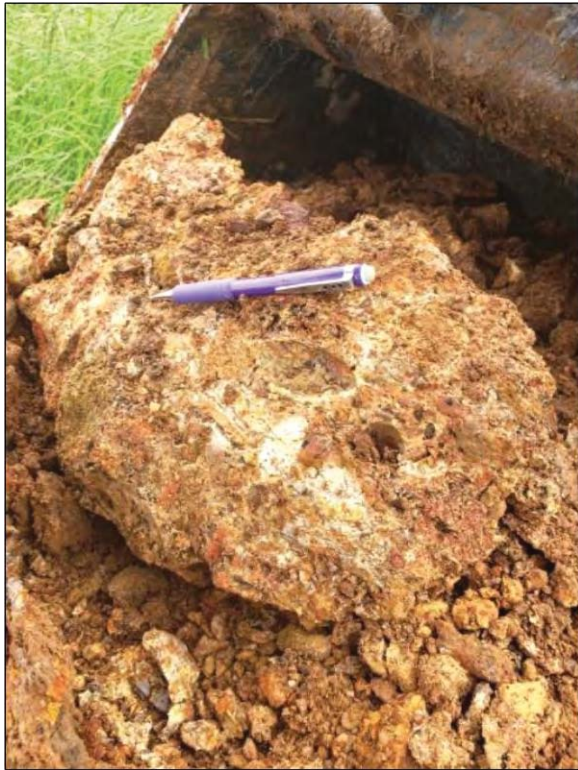
Photos TP-1: Test Pit TP-1 to approximately 13 feet in depth (below); Sample from bottom of exploration at 13 feet (left)
