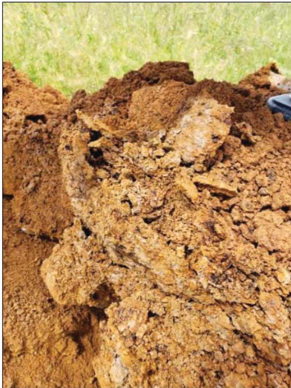
Photos TP-7: Test Pit TP-7 to approximately 9 feet in depth (below); Sample from bottom of exploration at 9 feet (left)
