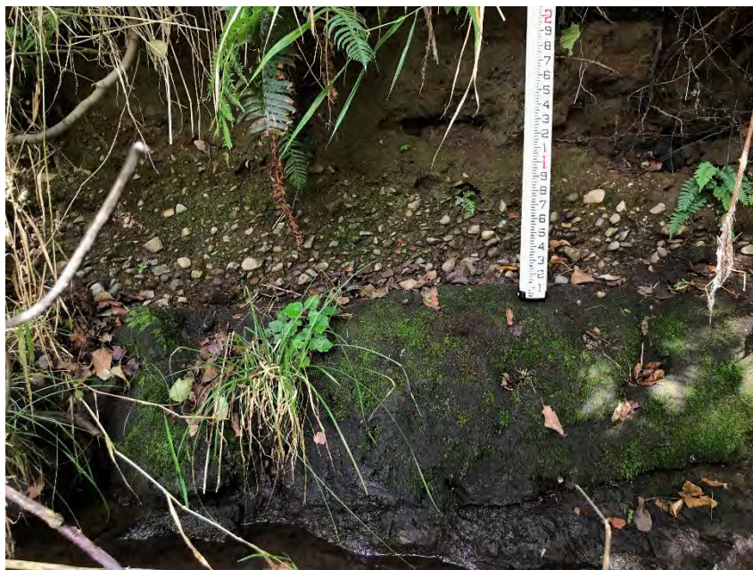
Figure 17: Exposed bank upstream of the stream crossing, showing mudstone bedrock at the base overlain with alluvium and forest soil (Station 28+20)
