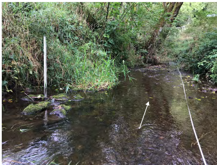
Figure 21 Channel conditions at the transition from the culvert outfall area to the confined reach just downstream of a sharp channel bend (Station 26+70, white arrow indicates flow direction)
