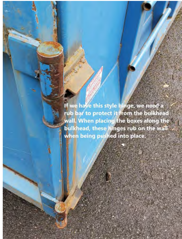
Figure 1: Non-Preferred Hinge Configuration
