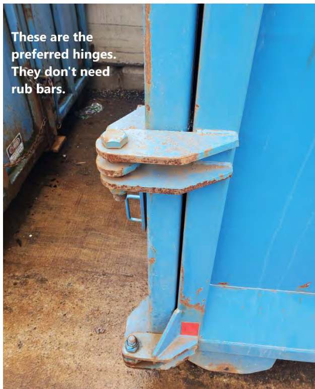
Figure 3: Preferred Hinge Configuration
